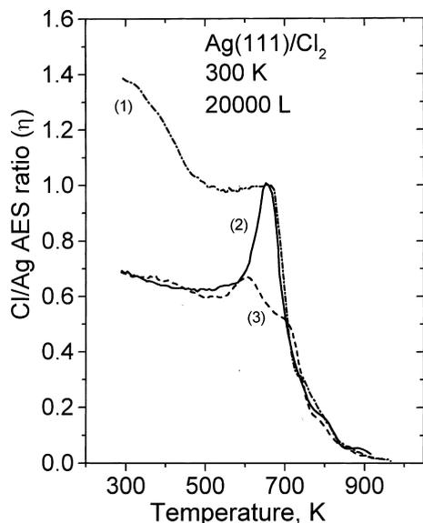
Fig. 8. Temperature dependence of Auger lines Cl  $L_{2,3}VV/Ag M_{4,5}VV$  intensity ratio with a linear heating rate of  $3.7 \text{ K s}^{-1}$  obtained for different primary current densities of 3-keV electrons. 1: measurement with  $\rho = 0.25 \mu\text{A cm}^{-2}$ ; 2: preliminary action at 300 K with  $\rho = 12.4 \text{ mA cm}^{-2}$  during 2 min, measurement with  $\rho = 0.25 \mu\text{A cm}^{-2}$ ; 3: measurement with  $\rho = 12.4 \text{ mA cm}^{-2}$ .
