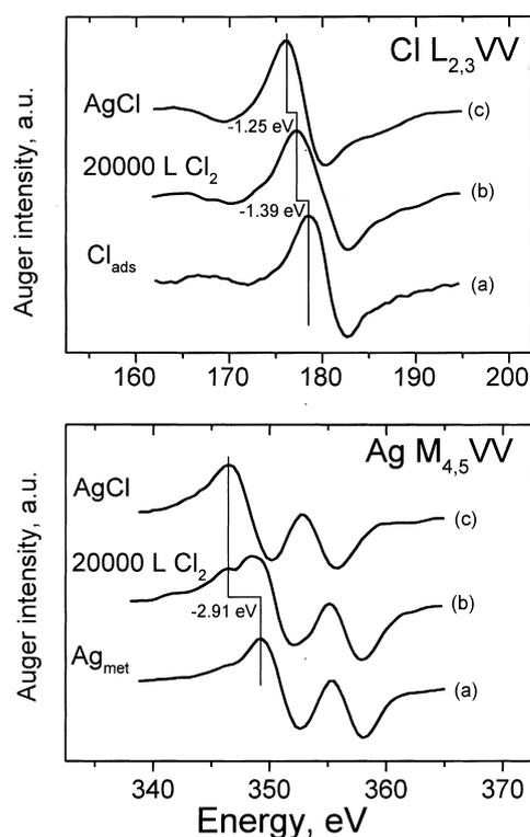
Fig. 3. Cl  $L_{2,3}$ VV and Ag  $M_{4,5}$ VV AES lines of chlorinated Ag(111) surface: (a) covered by a chlorine monolayer; (b) AgCl island film, 20 000 L dose of chlorine at room temperature; (c) AgCl continuous film.
