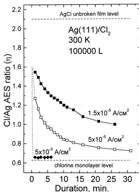
Fig. 7. Time dependence of the Cl  $L_{2,3}VV$ /Ag  $M_{4,5}VV$  intensity ratio under a primary electron action of 3-keV energy obtained for different electron beam densities. The lines in the range inaccessible for measurements are drawn by dotted curves. The signal level for monolayer coverage and that for the continuous chloride film are shown by dashed horizontal lines.
