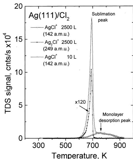
Fig. 4. Thermal desorption spectra of a chlorinated Ag(111) surface.  $\Delta$ :  $\text{AgCl}^+$  ion, chlorine monolayer coverage, 10 L;  $\square$ :  $\text{AgCl}^+$  ion, AgCl island film, 2500 L;  $\bullet$ :  $\text{Ag}_2\text{Cl}^+$  ion, AgCl island film, 2500 L.
