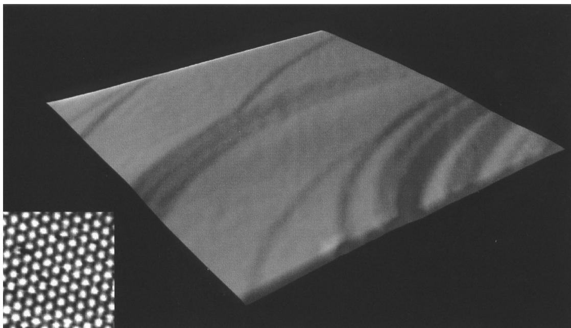
Fig. 1. STM image ( $7100 \times 7100 \text{ \AA}^2$ ) of a clean  $\text{Ag}(111)$  surface. Insert: atomic resolution image of  $\text{Ag}(111)$ - $(1 \times 1)$  structure,  $26 \times 28 \text{ \AA}^2$  ( $U_t = 50 \text{ mV}$ ,  $I_t = 1 \text{ nA}$ ). The interatomic distance is  $3.0 \pm 0.15 \text{ \AA}$ .
