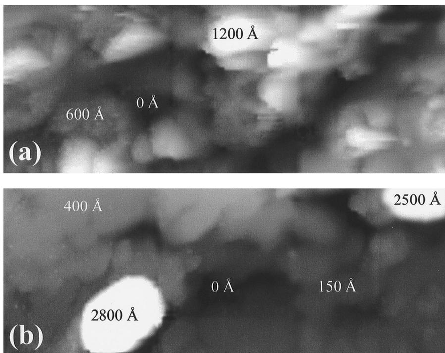
Fig. 6. STM image of Ag(111) surface chlorinated with a 100000-L dose of  $\text{Cl}_2$ .  $20800 \times 7800 \text{ nm}^2$  (a) before electron action and (b) after electron action of  $0.1 \text{ C cm}^{-2}$  dose ( $U_t = -1.5 \text{ V}$ ,  $I_t = 0.2 \text{ nA}$ ). (Different parts of the surface are shown.) The heights of the features are indicated.
