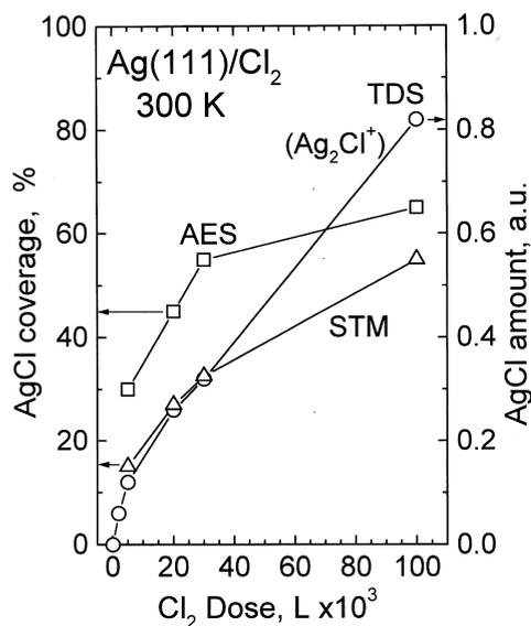
Fig. 5.  $\text{Cl}_2$  dose dependence of AgCl coverage measured by STM ( $\Delta$ ), AES ( $\square$ ) and AgCl amount measured by TDS ( $\circ$ ).
